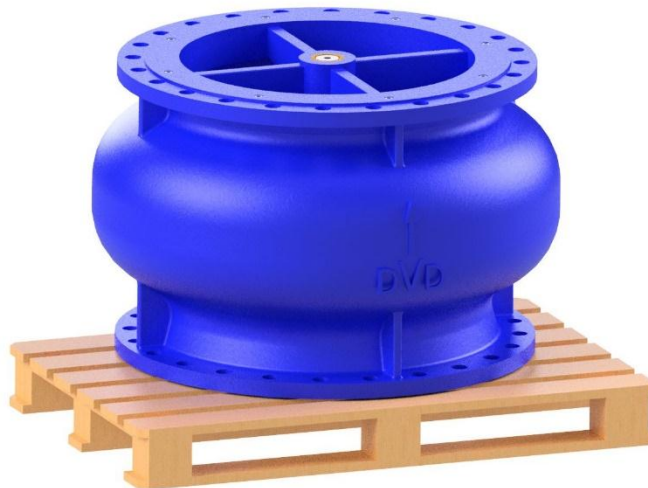
PICTURE 1: Positioning the Valve on the Pallet - In order to prevent damage to the seat and seal during transportation the disc of check valve should be positioned to be at the bottom
